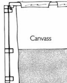
**Note:** When you insert the bottom horizontal poles into the verticals you must invert them so that the wedges face upwards. As per the diagram above. This is essential so that the poles hold the wall material taut. If you experience difficulty with connecting the poles, move over the material away from the corners to ease the tension. Connect the frame and stretch the material back into position.
